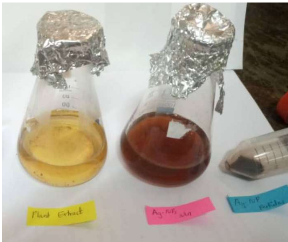
Figure 1. Aqueous Leaf Extract, Aqueous Synthesized C-Ag NPs and its Solid Synthesized C-Ag NPs.
