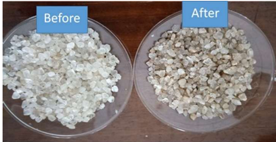
Figure 8. Presenting Natural Silica Sand Before and After Immobilization with Ag NPs. Source: Authors
